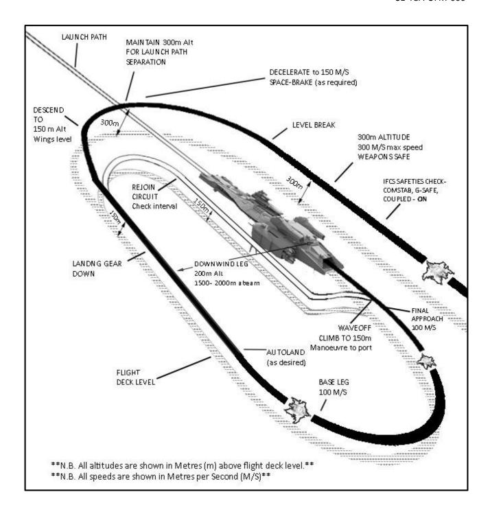
Figure 6-2 Carrier landing pattern
