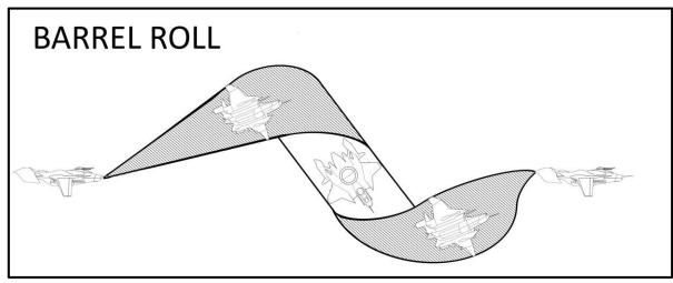
Figure 7-3 Barrel roll
