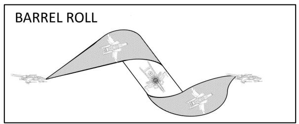
Figure 7-3 Barrel roll
