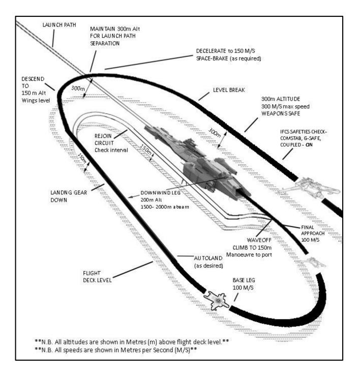
Figure 6-2 Carrier landing pattern
